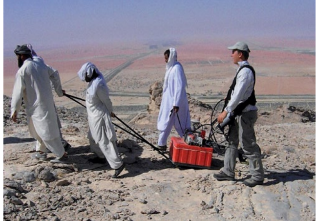
GPR measurement to explore ground water
